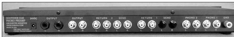
PHOTO 2: Rear panel of the EQS MK12. The ¼” jacks on the left are fully-balanced, tip-ring-sleeve outputs. RCA connectors are gold-plated and Teflon®-insulated. The jacks marked “Return 1” are actually the line inputs, which are placed ahead of the equalization circuits.
