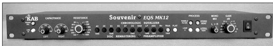
PHOTO 1: The K-A-B EQS MK12. Twelve equalization curves accommodate records from early acoustics through RIAA stereophonic discs. Adjustable cartridge loading, lateral-vertical switching, and a processor loop add to the unit’s flexibility.
