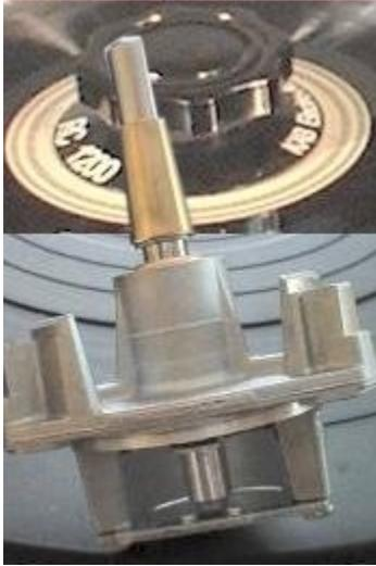
c) Integrated cartridge/head design with specific alignment for the SL-1200
